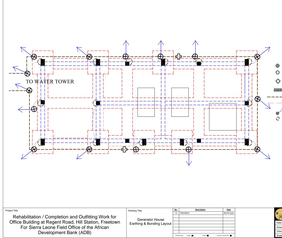
LEGEND Clamp: connecting copper conductor to earth rod cylindrical part, to be welded to steel structure or undation bars for using as connection point with cable shoe Clamp: connecting copper conductor to copper conductor or Y/G wire
